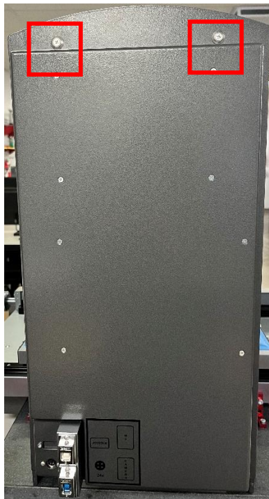
Figure 11. Accessing the MVR Rear Panel
