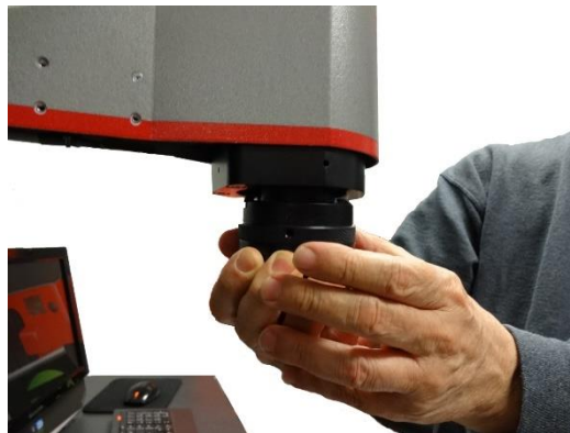
Figure 22. Removing the Optics Assembly
