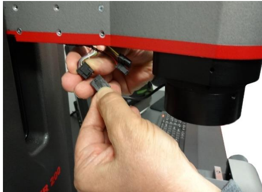
Figure 21. Unplugging the Ring Light Connector
