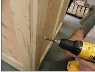
Figure 7. Removing the Screws from the Shipping Container
