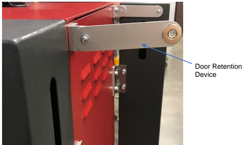
Figure 35. Magnetized Door Retention Device
