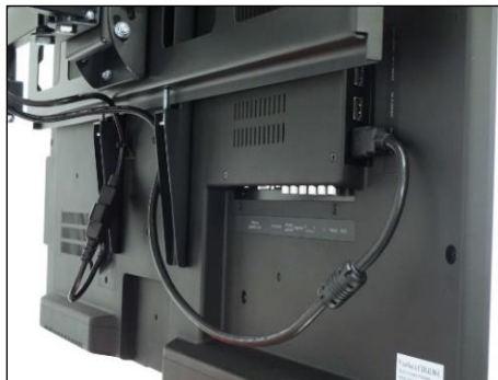
Figure 16. Video Monitor Cable Connections
