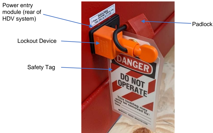
Figure 23. Installing the Lockout Device
