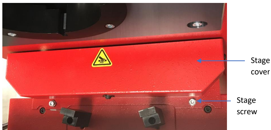
Figure 13. Y-Axis Stage Cover Screws
