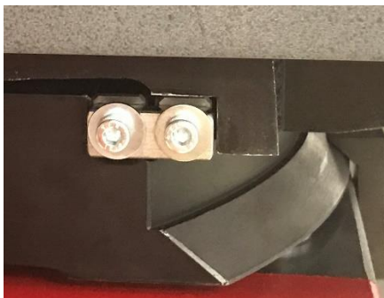
Figure 11. Z-Axis Stage Lock
