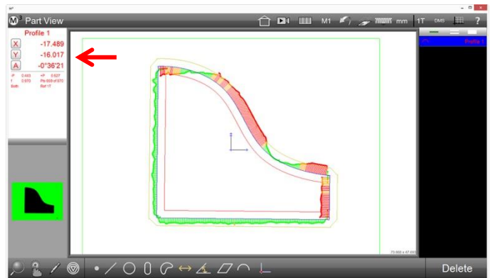
Profile measurement completed, results shown
