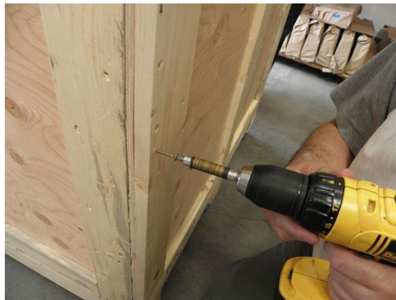
Figure 15. Removing Screws from the Shipping Container
