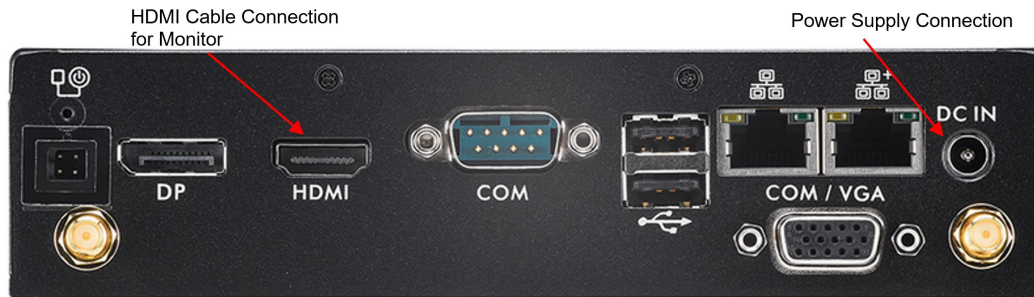
Figure 20. System PC Cable Connections
