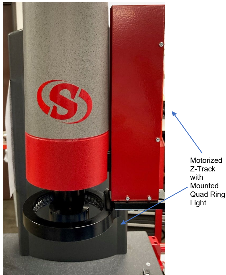
Figure 3. Motorized Z-Track with Mounted Quad Ring Light
