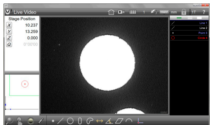
Failed tolerances are shown in red
