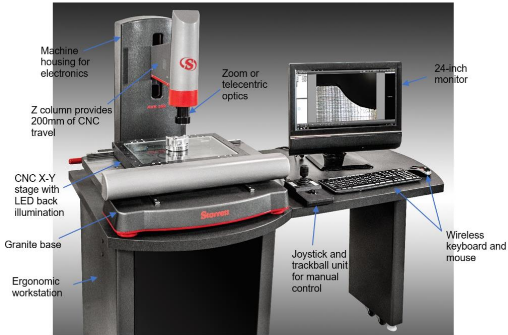
Figure 3. AVR System Components
