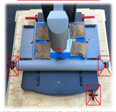
USE SHIPPING BAR TO LIFT MACHINE OFF OF CRATE, AS WELL AS THE TWO HANDLES IN THE REAR.
