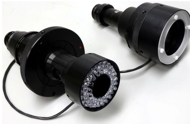
6.5:1 zoom optics assembly (left), telecentric optics assembly (right)
