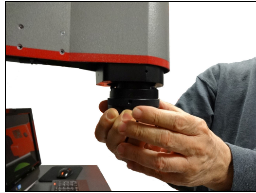
Then remove optics assembly using two hands.
