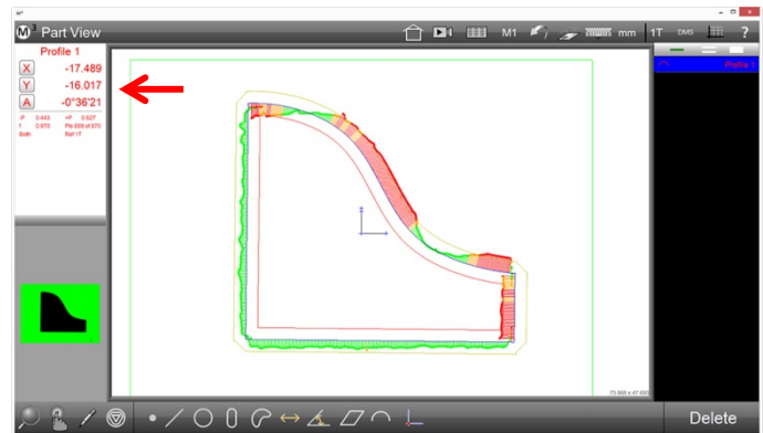
Profile measurement completed, results shown
