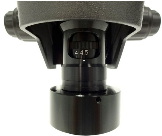
Knurled rotary control for zoom adjustment
