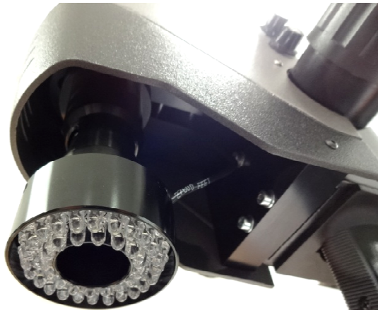
LED top illumination, controlled by knob at top of photo.
