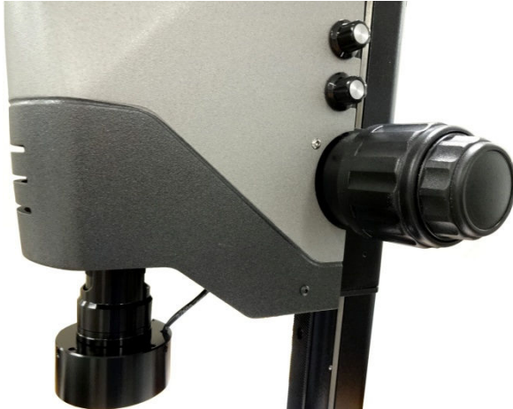
Brightness adjustment knobs (top) and height adjustment knobs (bottom)
