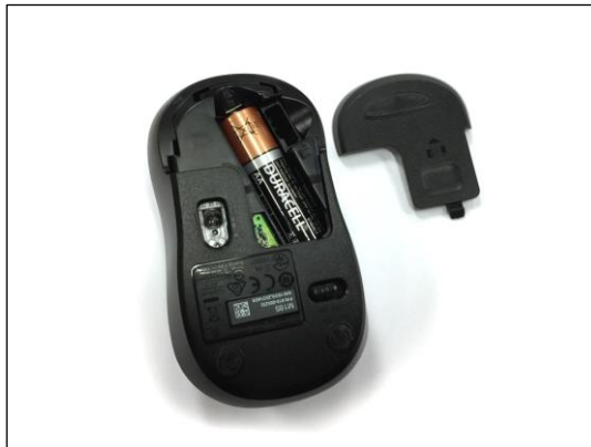
Wireless Mouse Battery Placement
