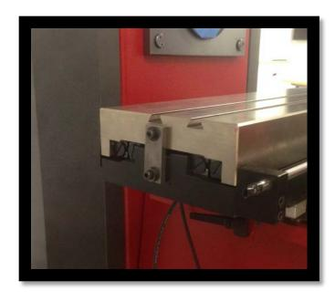
REMOVE THE STAGE LOCKS AND REINSTALL TWO
