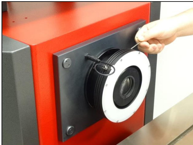
Figure 6. Removal and reinstallation of ring light.
