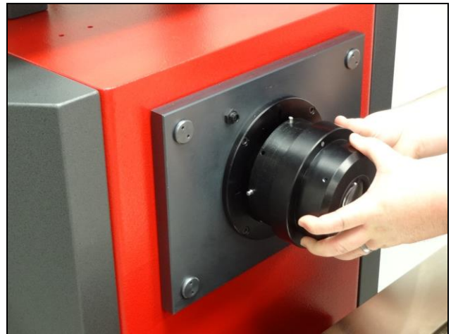
Figure 7. Removal and reinstallation of telecentric lens.
