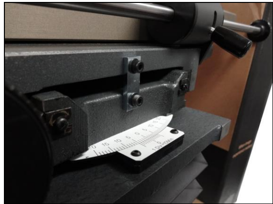
Figure 11. Removable shipping tab
