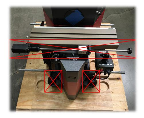
USE SHIPPING BARS TO LIFT MACHINE OFF OF CRATE.
