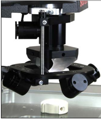
Figure 2 - 3: Quad lamp Illuminator in its dark field (or side) illumination position.
