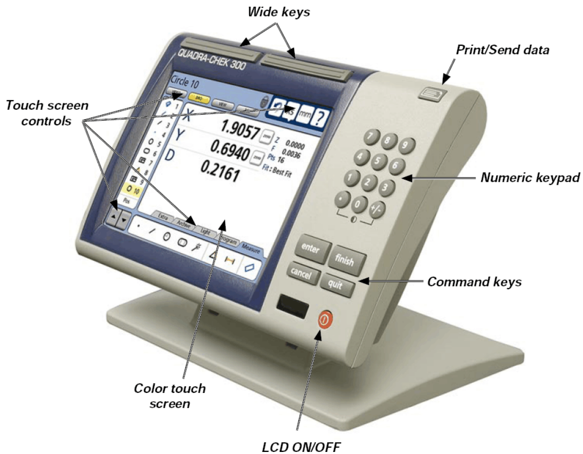
Figure 4 - 4: QC300 Main Controls
