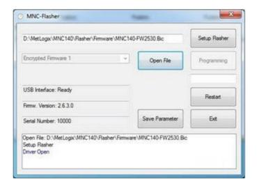
B) Flash the FPGA (MNC140-GA0012.Bic) with the single flasher
