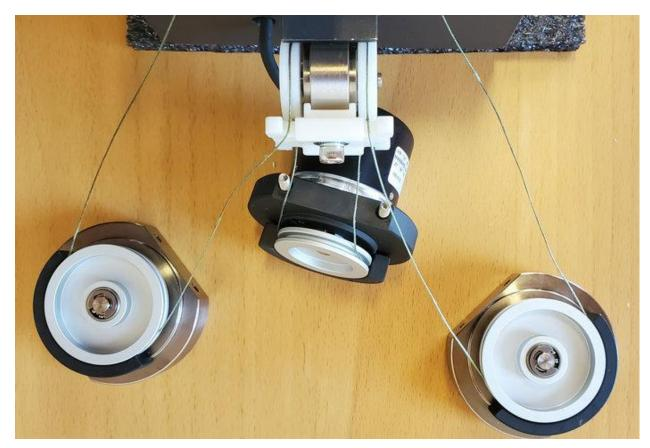
If the wire has come off the counterweight pulley(s), you may need to loosen the allen bolt on the top of that assembly in order to route the wire in the wheel channel(s). This bolt connects the weight (which also serves as the pulley guard) to the rest of the assembly. Re-tighten the bolt once the wire is correctly routed.
