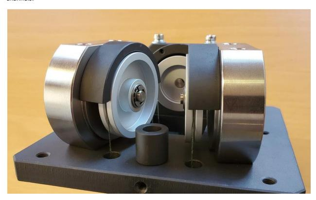
The guards over the tops of the wheels are there to help prevent the wire from coming off during normal operation, but it is still possible for the wire to pop off if the unit has been mishandled. If the wire has come off any of the pulleys, it should be possible to get it back on track without having to remove the guards (as there is a fine gap between the guard and wheel that the wire can squeeze through).
