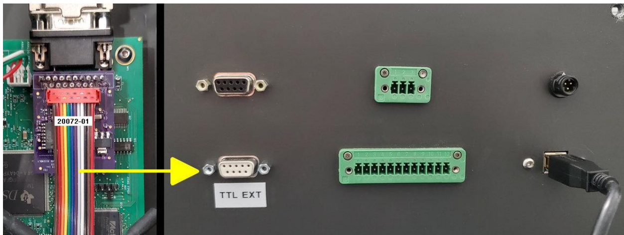
Extensometer cable installed in dual column test frame.
