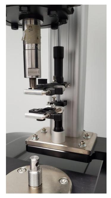
Move the crosshead down so that the starting point for the test is near the gage length (this distance is not critical, so do NOT travel too close and risk damaging the arms with a collision). It would be wise at this point to set the lower hardware limit switch on the stand so that the crosshead can not move further down and crush the extensometer arms.
