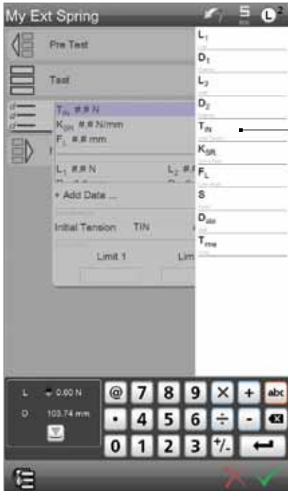
The Initial Tension coefficient (TIN) is only displayed when the Measure Initial Tension option is selected.
