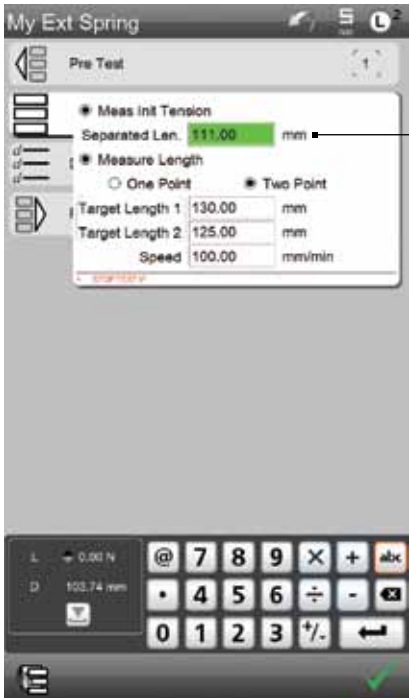
The Separation Length is the measured length of the spring when load is applied sufficiently to separate all coils from one another.
