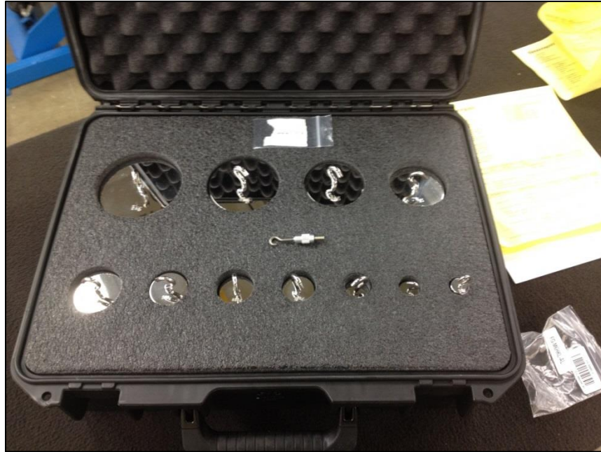
Figure 1: An example of a hanging deadweight kit
