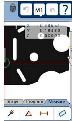
Adjust the contrast threshold by touching and sliding the yellow arrow
